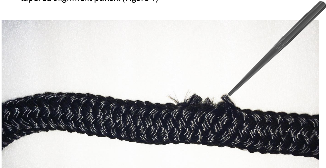
Figure 4: Repairing Damaged Rope Strands - 02
