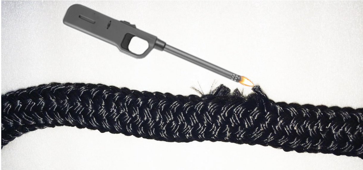
Figure 3: Repairing Damaged Rope Strands - 01
