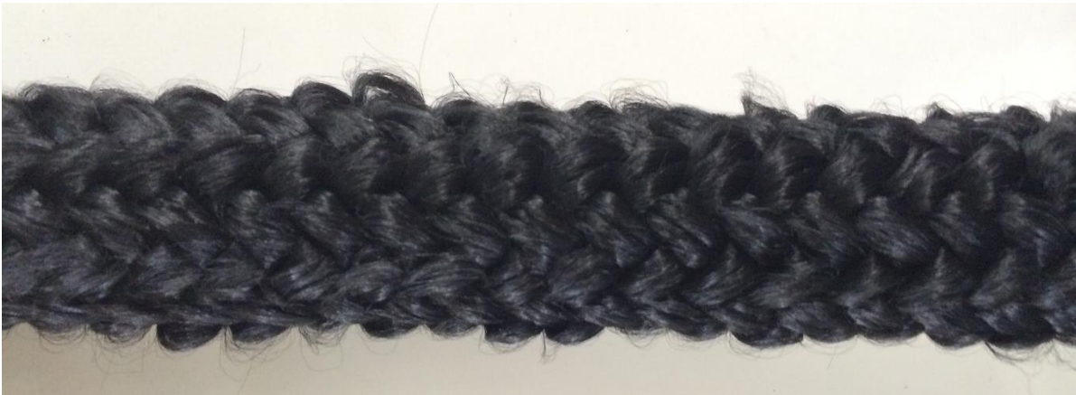
Figure 1: Polyester Black Rope with some signs of frayed fibers and strands
